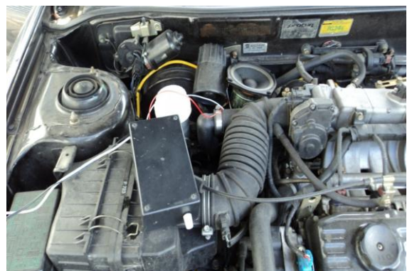
Fig. 3: Position of the loudspeaker as the substitution source to obtain exterior SPL.
