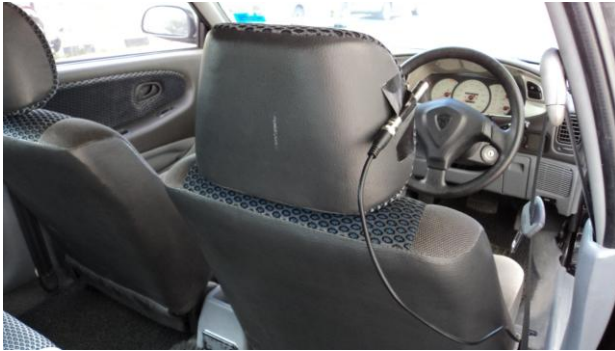
Fig. 5: Position of the microphone to measure interior SPL.
