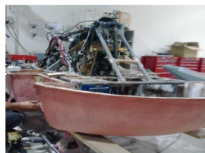
Figure 6: Assembly Process in Space Frame Chassis
