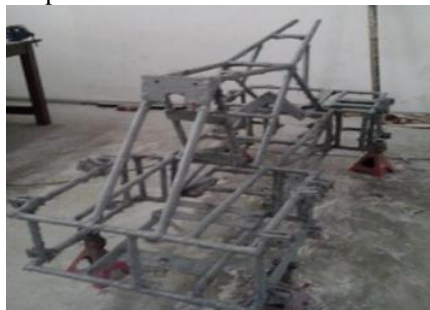
Figure 5: Joining Process of Chassis Fabrication
