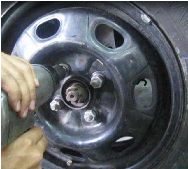
Fig. 11. Removing one wheel nut using impact wrench.
