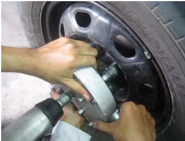
Fig. 12. Removing all wheel nuts using VAWNR and impact wrench.
