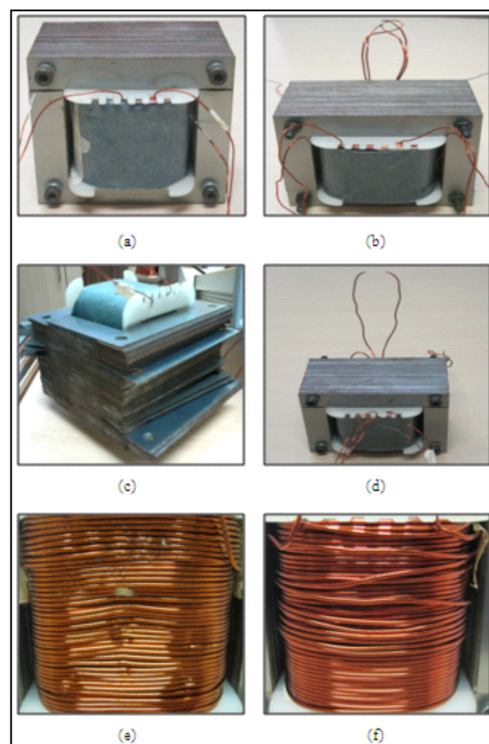
Fig. 4: Transformer Model for each faults (a) Healthy Transformer, (b) Shorted Turns, (c) Core Damage, (d) Open Circuit, (e) Radial Deformations and (f) Axial Displacements Fault.
