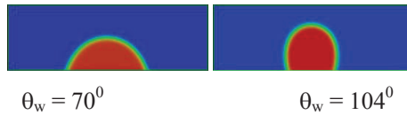
FIGURE 1: Droplet at equilibrium contact angle
