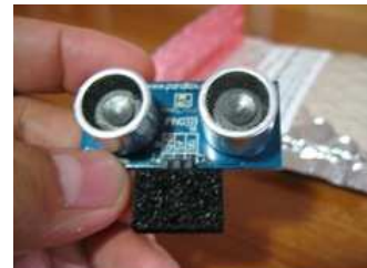
Figure 7: PING Ultrasonic Sensor Distance
