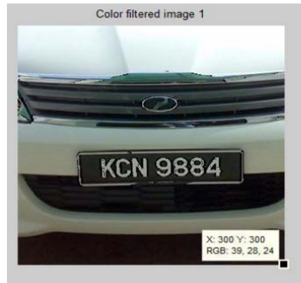
Figure 6: Result after filtering by using colour edge detection
