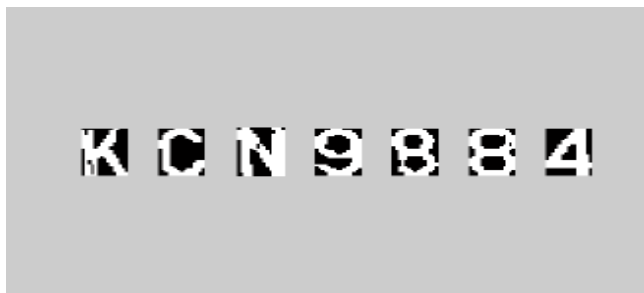
Figure 14: Final result obtained after character separation phase
