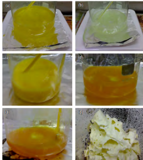
Fig. 1. Evolution of (a) Bi-Ti precursor (b) Pr precursor (c) Bi-Ti precursor stirred at 40°C for 2 hour (d) Bi-Ti precursor heated at 90°C (e) viscous gel and (f) as-combusted powder.
