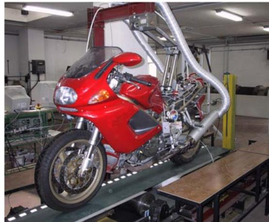
Fig. 1. Motorcycle on the FSMDR rig
