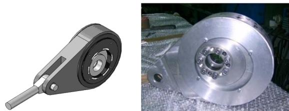
Fig. 2. Crank-rod drive mechanism
