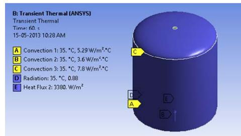
Fig. 1(b). Convection and radiation loads in thermal analysis
