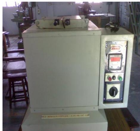
Fig. 1. Laboratory stir casting set up
