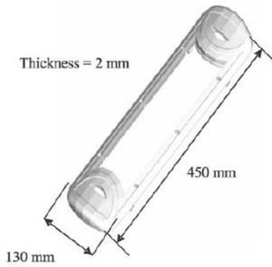
Fig. 25. Dimensions of bus ceiling lamp [36]
