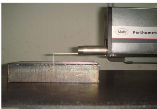
Fig. 1. Surface Roughness Analysis
