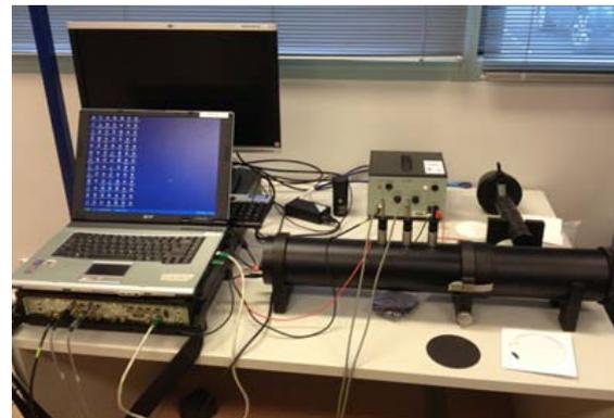
Fig. 2. Impedance tube set up
