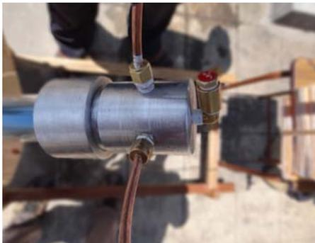
Fig. 5. Header in experimental set up
