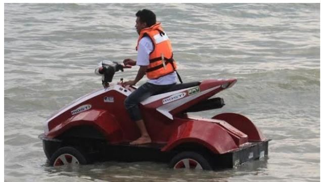
Fig. 3A. Complete AHV with hybrid propulsion system [12]
