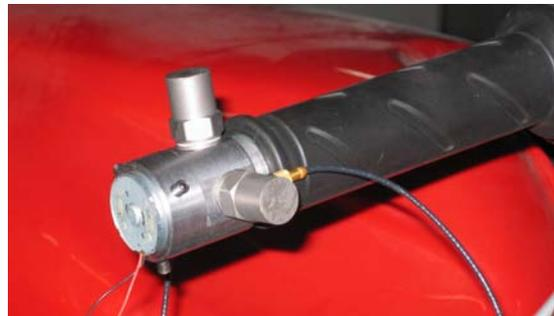
Fig. 2. Handlebar shaker/accelerometers
