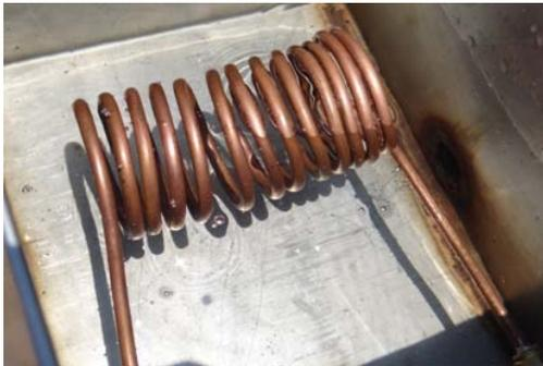
Fig. 3. Heating Coil
