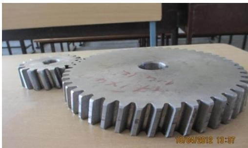
Fig. 3. Helical gear and Pinion for Steel C45
